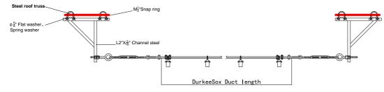
When bracket is fixed on girder of steel frame, there are some connection modes, such as hoop connection, bolt connection and welding, etc., and the bracket is generally quite long in direction, so we suggest the bracket be made of channel steel.
