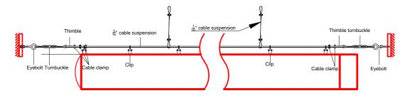
Schematic Drawing of Cable Installation System
